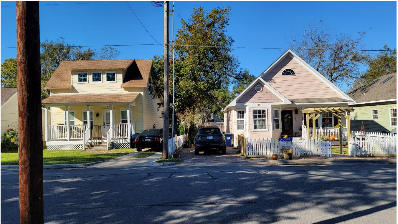
505 Hosea & Adjacent property to south- South home built in center of the lot- has driveway in zero-lot line area
